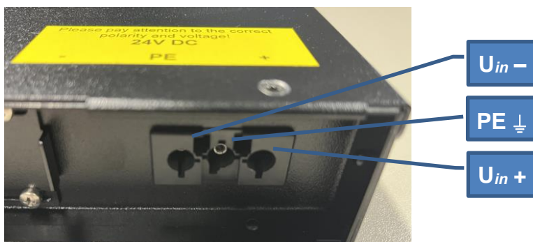
Figure 12: DC voltage connection at the power supply
