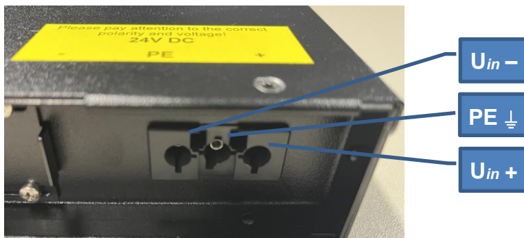
Figure 11: DC voltage connection at the power supply
