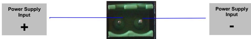
Figure 9: *Power supply input*
