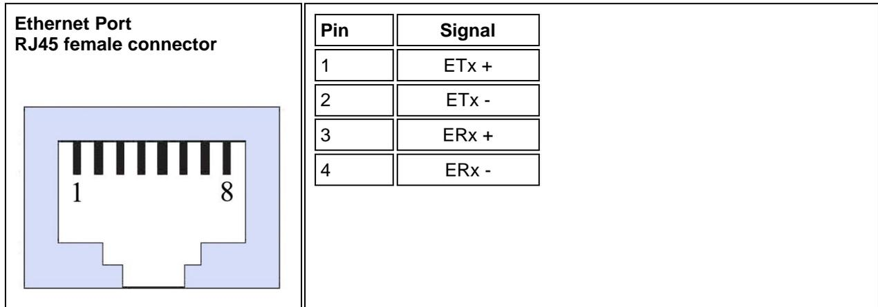
Figure 7: Pin assignment of Ethernet RJ45 interface
