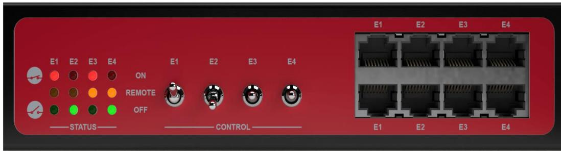
Figure 14: LEDs E1 – E4
