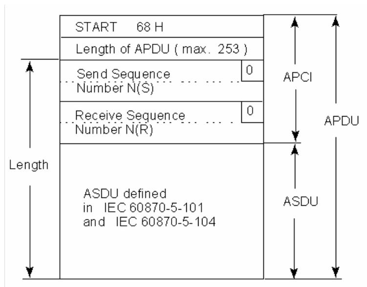
The message length is a maximum of 255 bytes with a maximum 249 bytes of ASDU.
