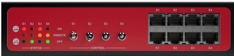
Bistable relays are used as "ON/OFF switches" for each of the eight individual lines of an Ethernet connection. These retain their current state even after a power failure or an interruption in communication. A one-to-one pin allocation is applied to connect or disconnect the partner interfaces.
